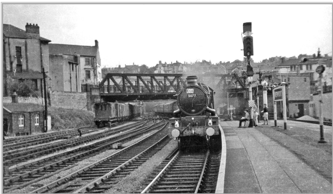
A trio of youthful spotters witness 'Castle class' No.5077 Fairey Battle enter the island platform circa 1962 with an express to Paddington. The Landore-based loco has its customary silver-painted buffers, a distinctive feature applied by the Swansea shed. The newly installed MAS signalling is in evidence on the platform during what would have been a transition period in the Newport Area Resignalling scheme.
